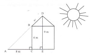
4. In the following diagram, triangles ABC and ADE are similar. The measurements are given in metres. What is the measure of segment EC, rounded to the nearest hundredth of a metre?
